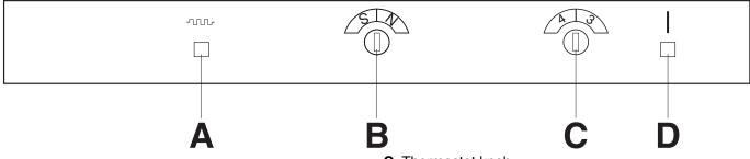
A. Pilot light for ambient temperature switch
